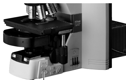
Turn the field diaphragm knob and stop down the field diaphragm to its minimum setting.
