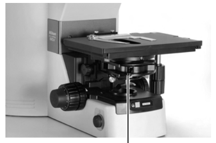
Aperture diaphragm lever (When using a condenser other than the motorized universal condenser)
